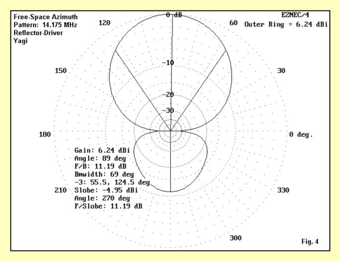
The 11 dB front-to-back ratio is a big improvement over initial parasitic design. Notice that to achieve this value, we had to lengthen the reflector considerably. At the same time, we shortened the driven element to restore it to resonance. The feedpoint impedance of this model is 34 Ohms with no reactance's typical figure for antennas of this general design.
