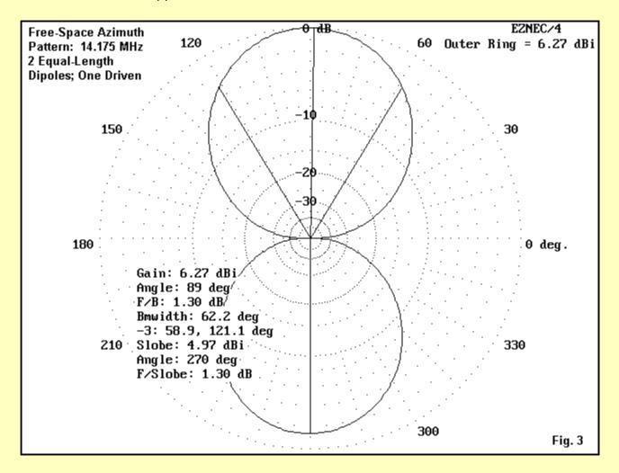
First of all, we get an antenna pattern that looks like **Fig. 3**. With a front-to-back ratio of only 1.3 dB, there is not much beam action. However, notice the gain value: nearly 6.3 dBi. The gain comes from the fact that part of the energy of the driven element is coupled to the undriven element, which then radiates that energy. Part of that energy contributes to the combined radiation that gives us the gain.
