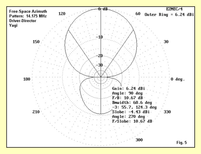
At the spacing we have selected, the performance of the antenna is almost identical to the performance of the driver-reflector design at 14.175 Mhz, asshown in **Fig. 5**. The relative current on the director is 0.75 with a phase angle of -146 degrees. That is equivalent to having a phase angle of 0 degrees on the forward element and an angle of 146 degrees on the rear element.
