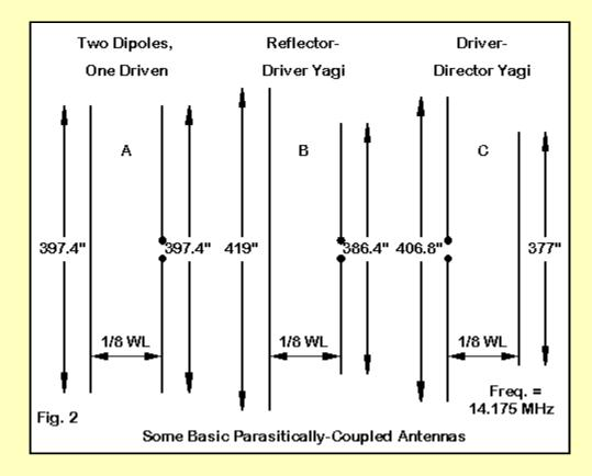
Now, let's go to **Fig. 2**, where we feed only one of the two elements. We shall once more begin with the left-most antenna design, which again uses our two original dipoles. However, only one of
