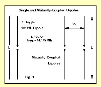
Let's begin with the simple dipole, the left-hand sketch in **Fig. 1**. The dipole we shall use as our example is set for 14.175 Mhz and uses 1" diameter aluminum tubing. All the rest of the antennas we shall look at use the same frequency and the same material. However, the principles apply to any dipole of any material on any band. Since we are working on general principles, we shall place our antennas in free space as an environment.
